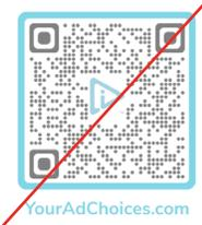
Don't forget to add a four-module space between the code and the frame.
